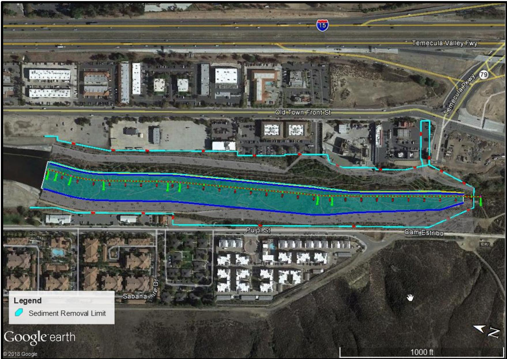
**Figure 3.** Area of Sediment and Vegetation Removal in Phase I of the Project. The area represented in blue are the limits of ground disturbing work within the channel. Note the unmaintained channel will not be impacted by this action.
