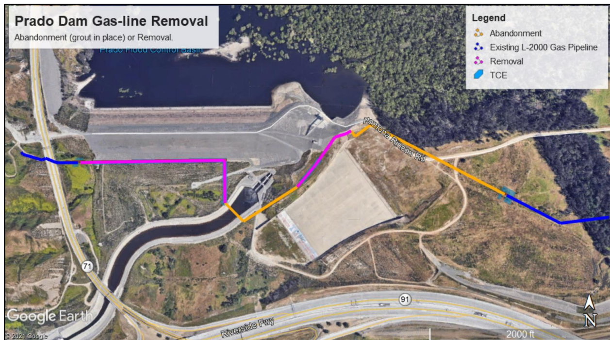
Figure 3. Proposed Grout in Place and Gas-line Removal
