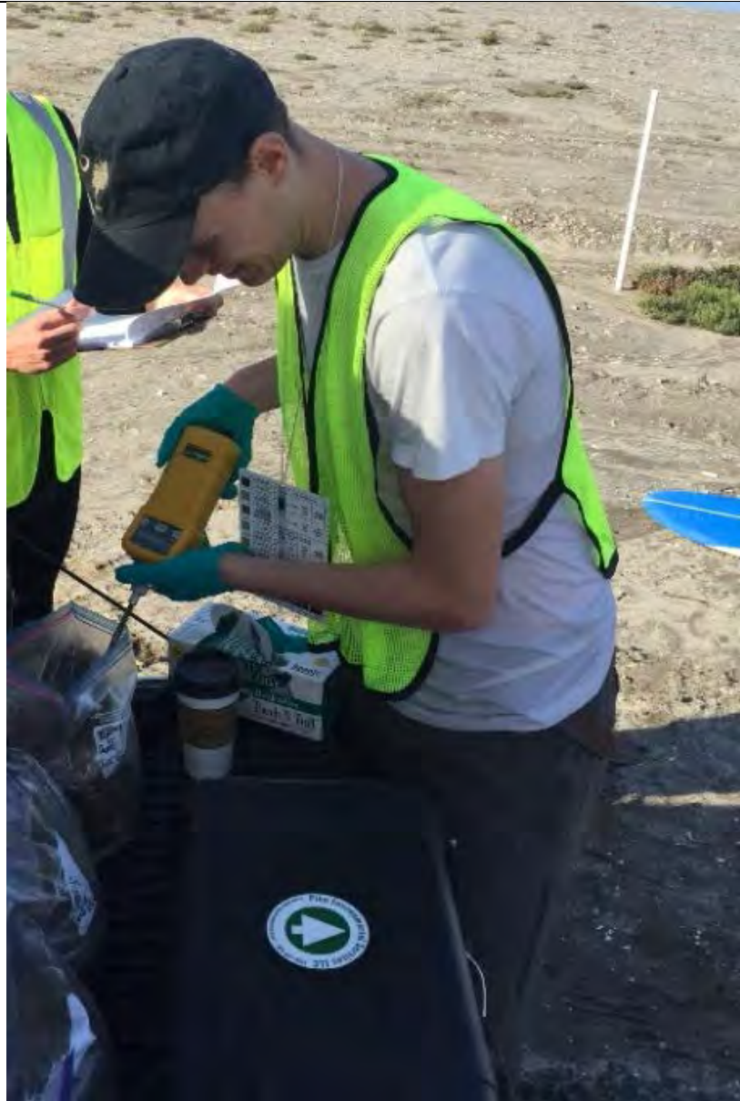
PID MiniRae Volatile Organic Compound Testing
