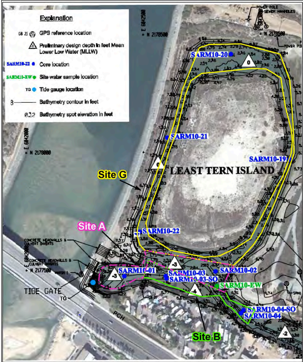
Figure 8. USACE 2012, SAR Marsh Relevant Borings
