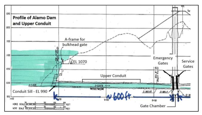
Figure 2. Profile of the Alamo Dam showing the bulkhead gate A-frame, upper conduit, and gate chamber.
