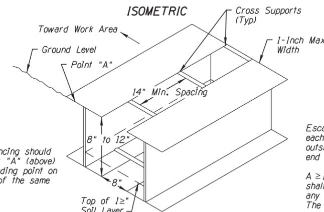
Parallel "1" beam are welded, using cross supports to maintain in 8" spacing, to create the tortoise guard.
