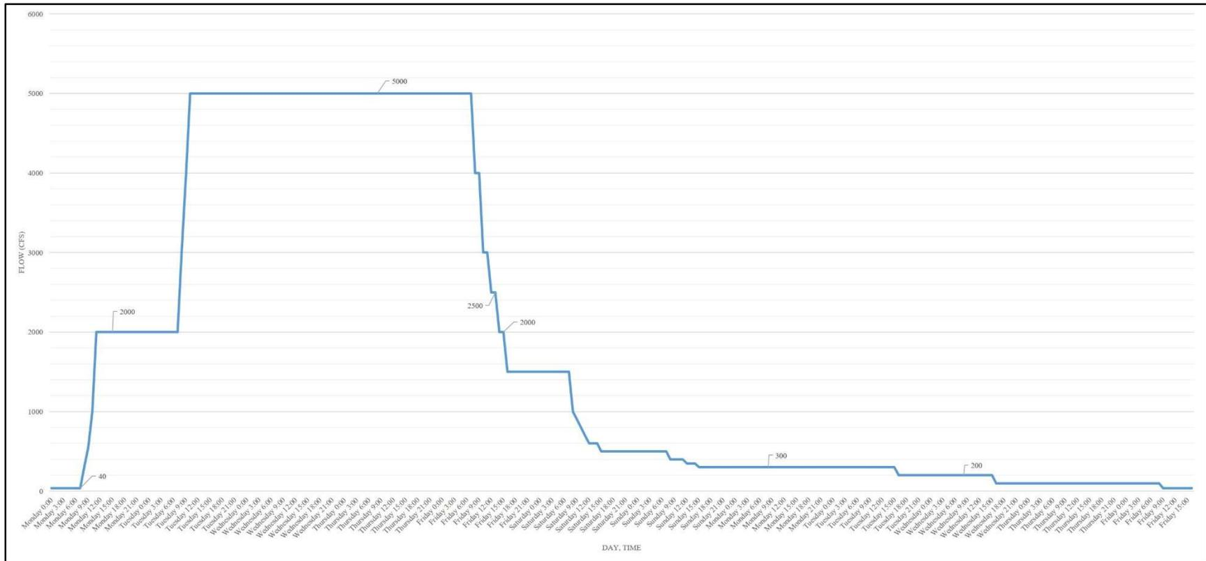
**Figure 2.** Conceptual hydrograph illustrating shape of the proposed release.
