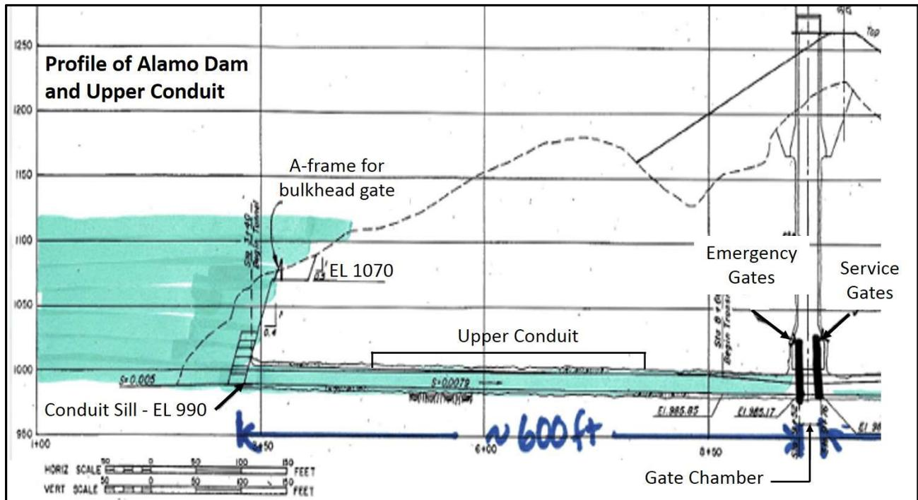
**Figure 2.** Profile of the Alamo Dam showing the bulkhead gate A-frame, upper conduit, and gate chamber.
