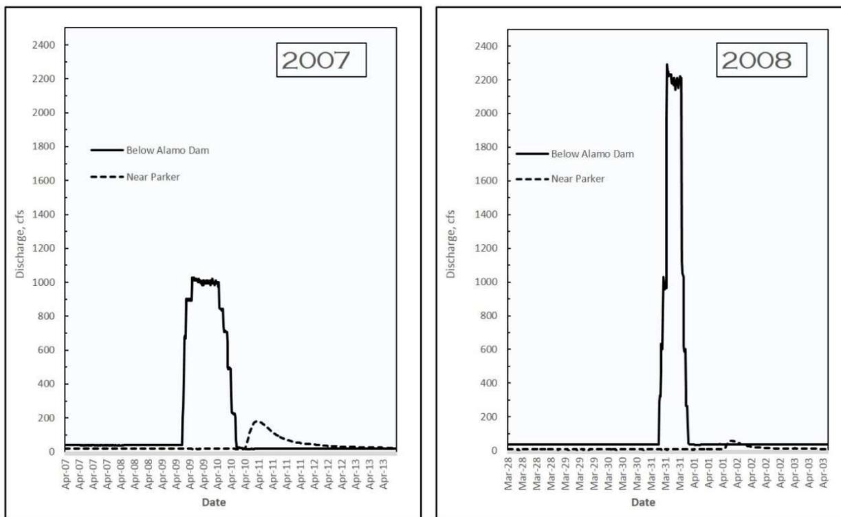
**Figure 14.** Flow attenuation from two pulsed releases from Alamo Dam in 2007 and 2008; the same events as reported in Andersen et al. 2010.
