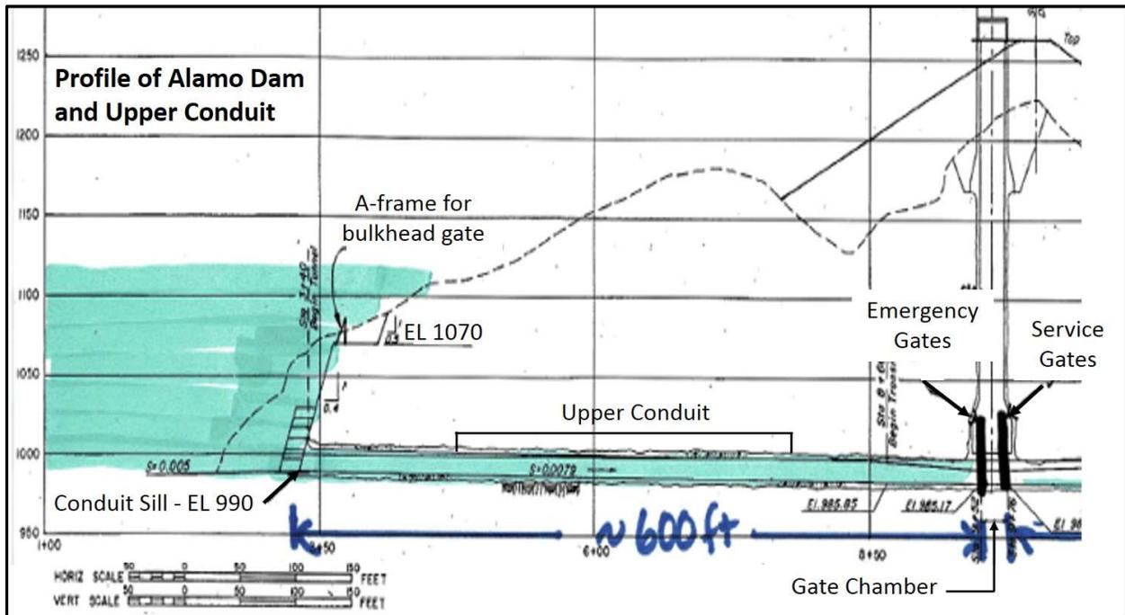
**Figure 1.** Profile of the Alamo Dam showing the bulkhead gate A-frame, upper conduit, and gate chamber.
