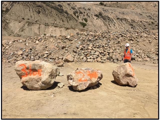
Figure F. 3-ton, 2-ton and 1-ton quarry rocks arranged left to right.
