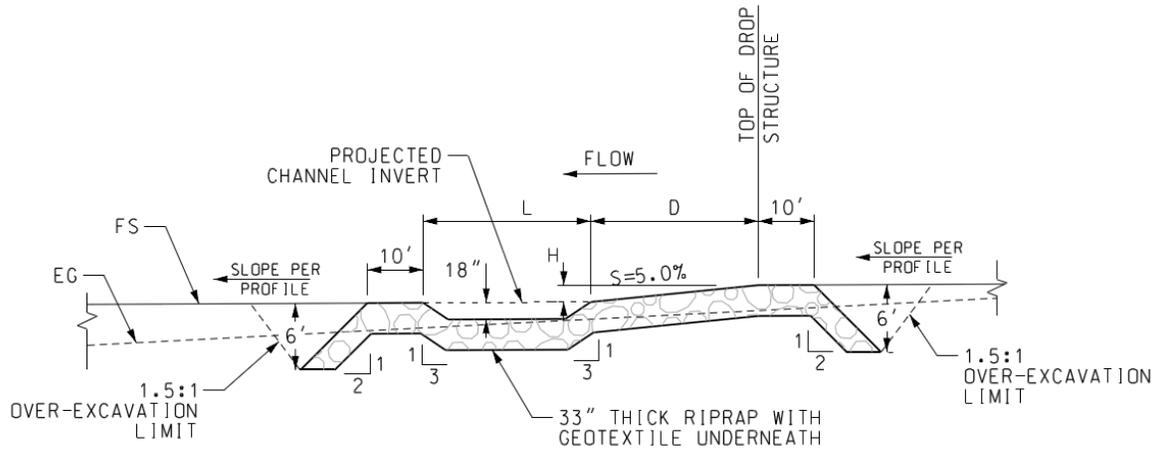
RIFFLE STRUCTURE DIMENSIONS
