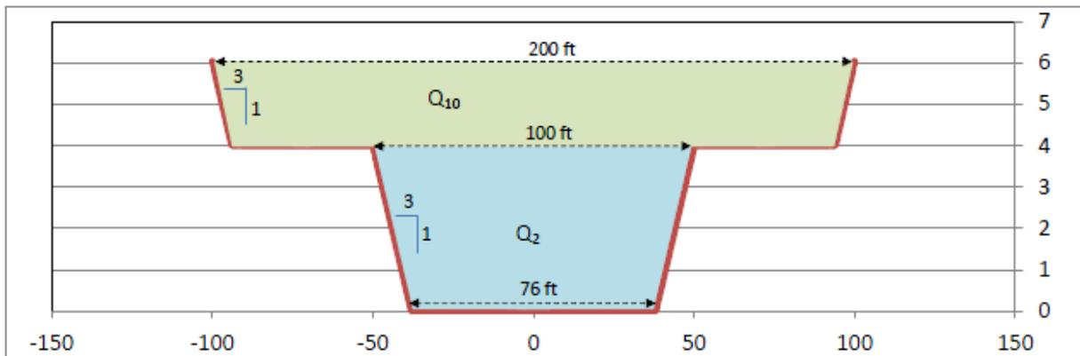
Figure 2.2 – Design Channel Template in Alternatives 3 and 4
