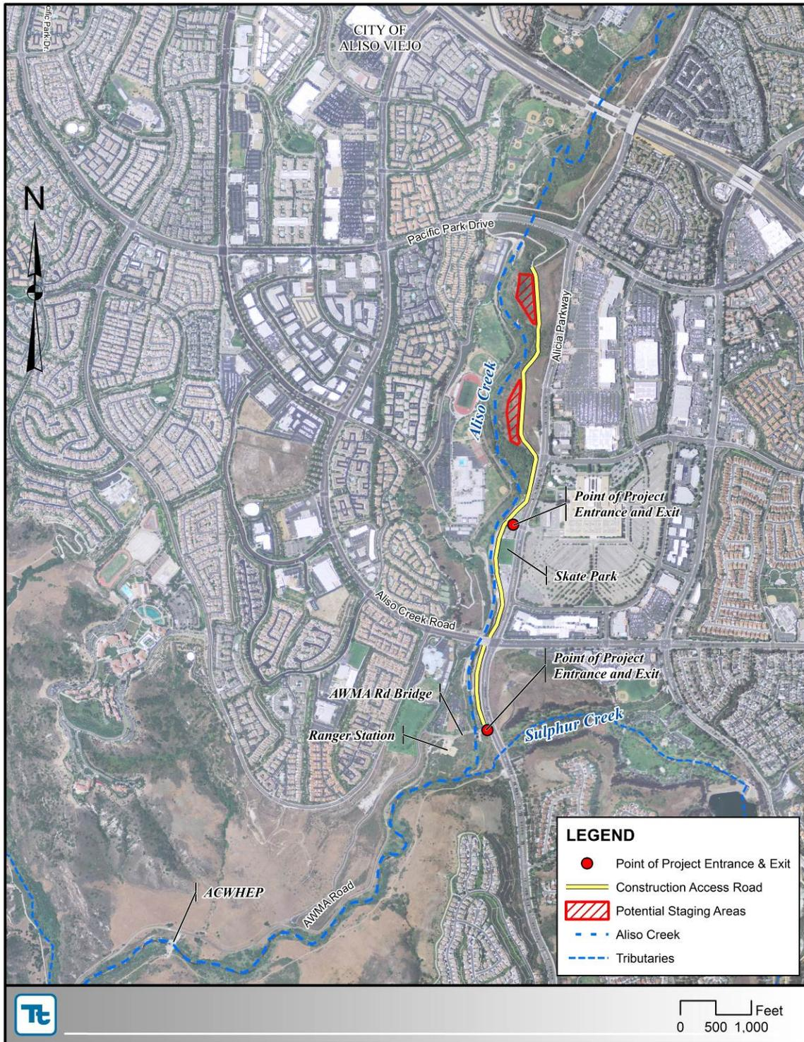
Figure 4.2 – Construction Access Road and Staging Areas (Upstream of AWMA Road Bridge)
