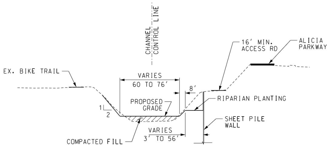
**Figure 3.8 – Typical Channel Widening near Aliso Creek Road Bridge**
