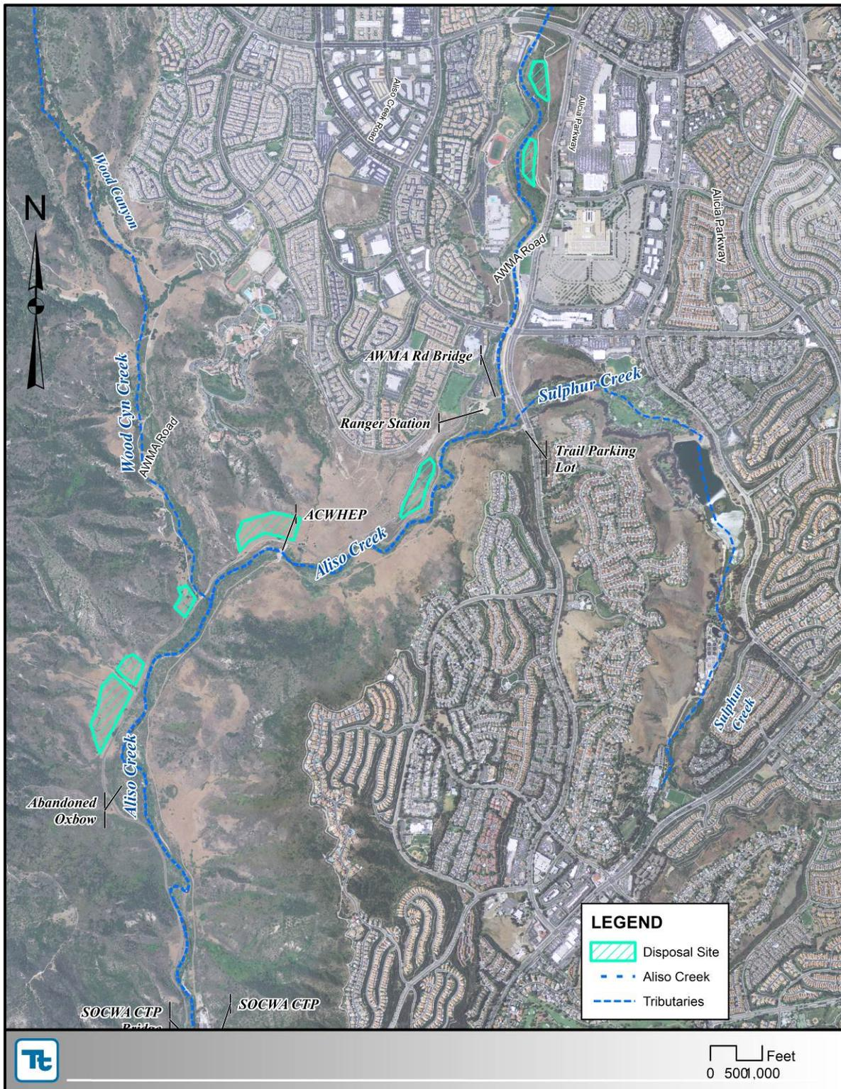
Figure 3.10 – Potential Disposal Sites for Excess Material
