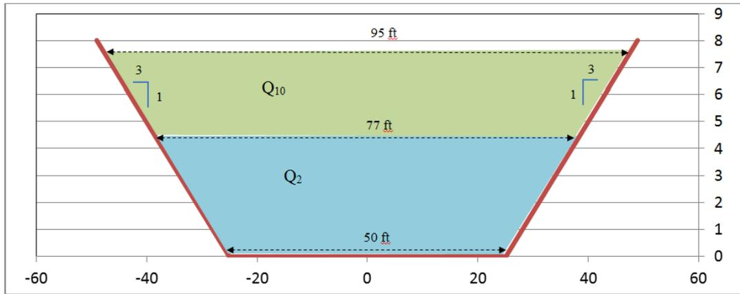
Figure 2.1 – Design Channel Template in Alternative 2
