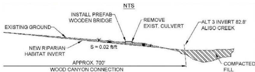
**Figure 3.7A – Profile along Wood Canyon Creek from Addendum Design (USACE 2017)**
