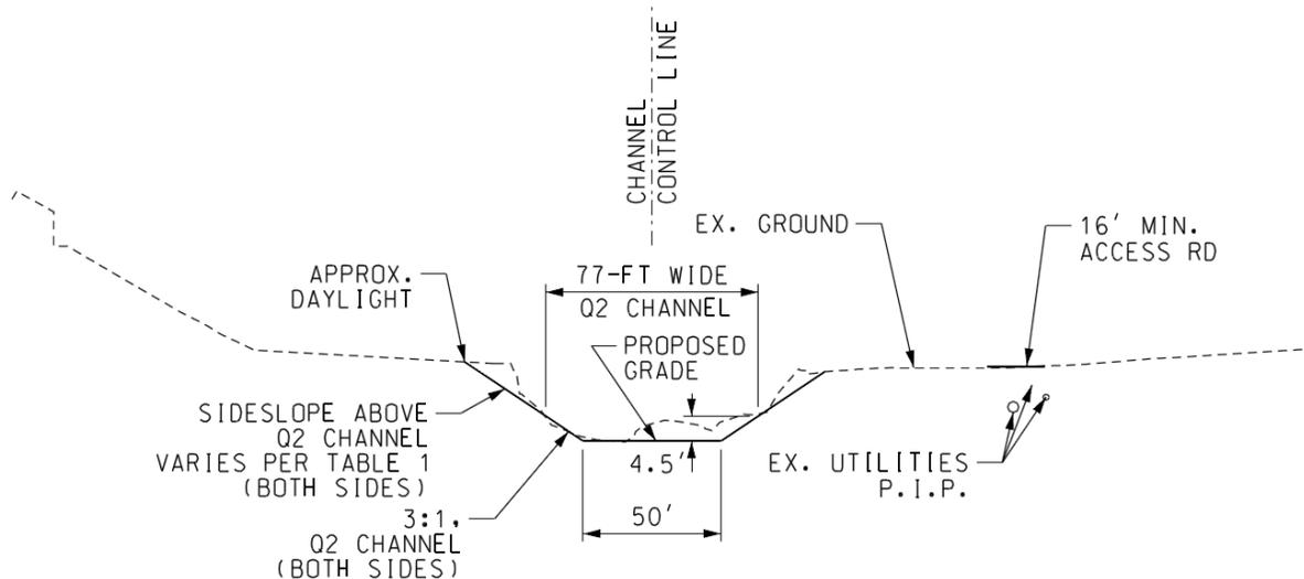
**Figure 3.1 – Typical Channel Design Section (Alternative 2)**
