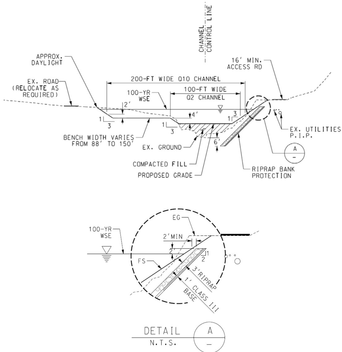
**Figure 3.4 – Typical Channel Design Section at Protected Bends (Alternatives 3 and 4)**
