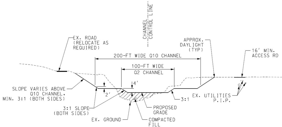
**Figure 3.3 – Typical Channel Design Section (Alternatives 3 and 4)**
