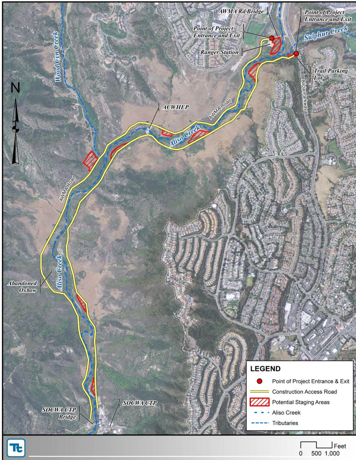
Figure 4.1 – Construction Access Roads and Staging Areas (Downstream of AWMA Road Bridge)
