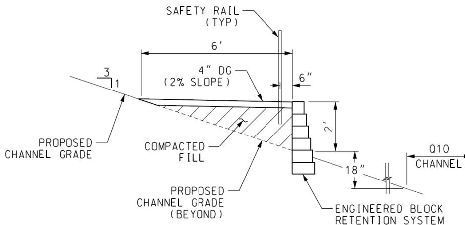
**Figure 3.5 – Typical 6-Foot-Wide Decomposed Granite Road with Retaining Wall**
