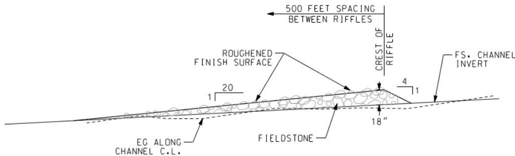
**Figure 3.9 – Typical Newbury Riffle Structure (Profile View)**
