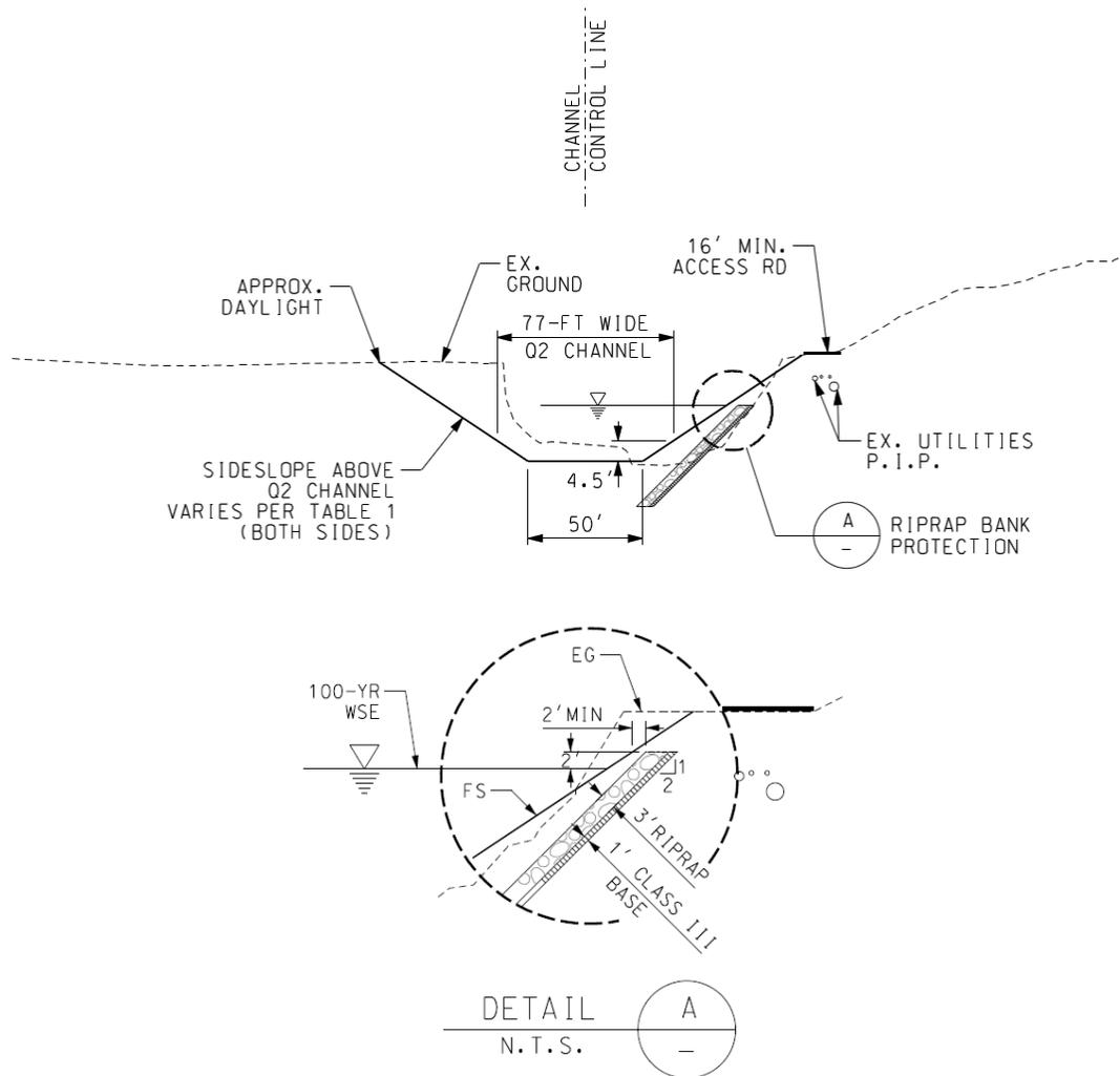
**Figure 3.2 – Typical Channel Design Section at Bends (Alternative 2)**
