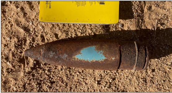
Top: 2.75-inch practice rocket warhead removed from site
