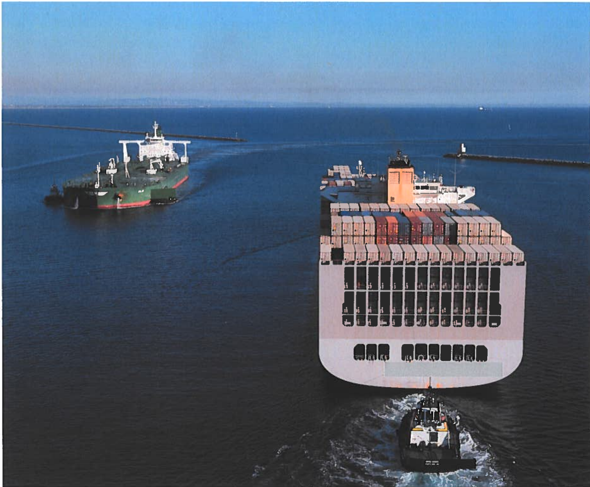
Very large crude oil carrier inbound Long Beach and very large container ship outbound, both in the wave shadow of the middle and east breakwaters. These very deep draft ships need flat water, provided by the breakwaters, to safely transit without touching bottom.
