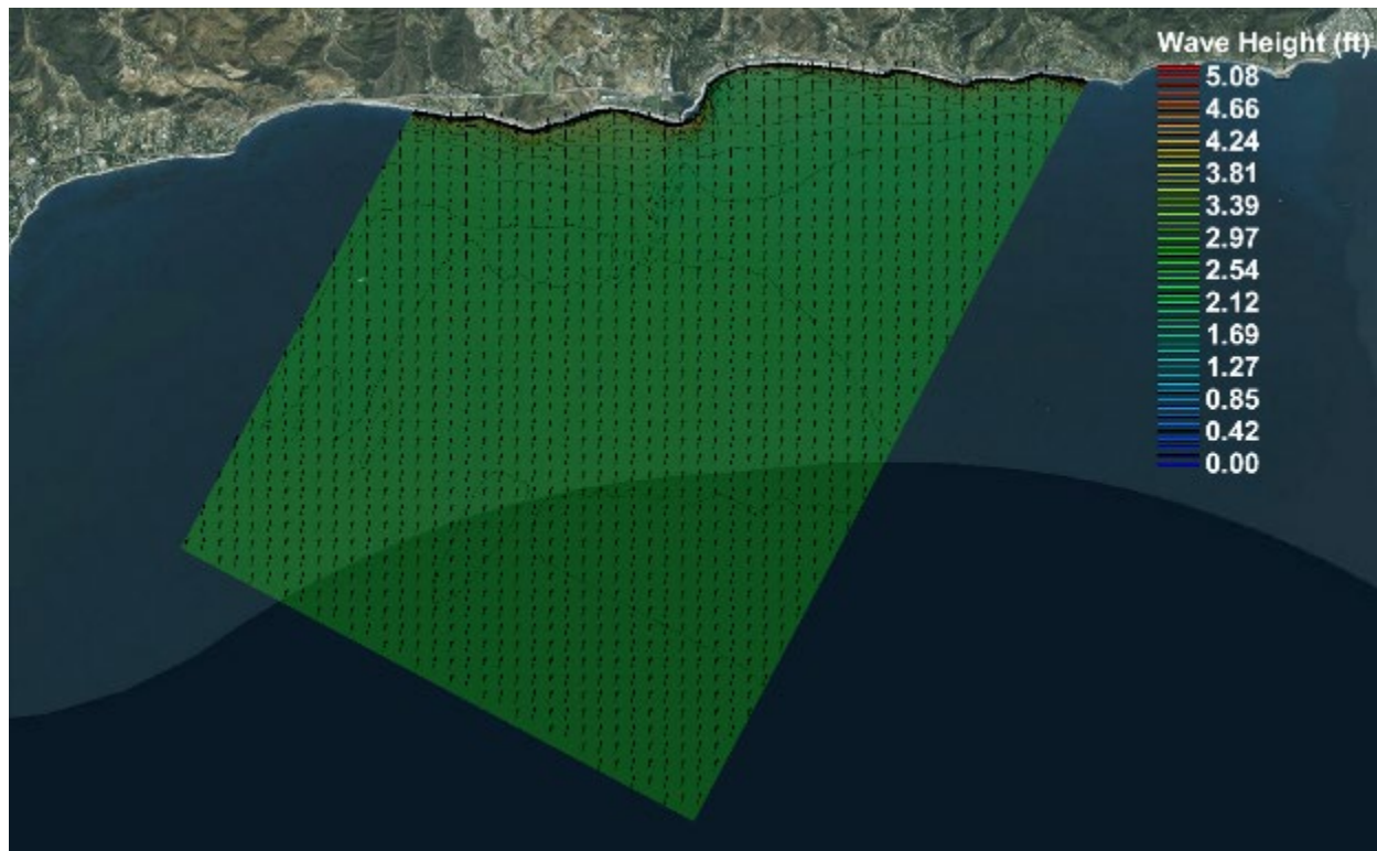
Figure 4.1-2: Typical conditions of project location ( H_s=2.75 ft, T_p=14 s, D_p=195^\circ )
