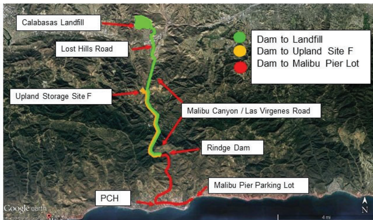
Figure ES.7-1 – NER Plan – Hauling and Placement of Rindge Dam Impounded Sediment
