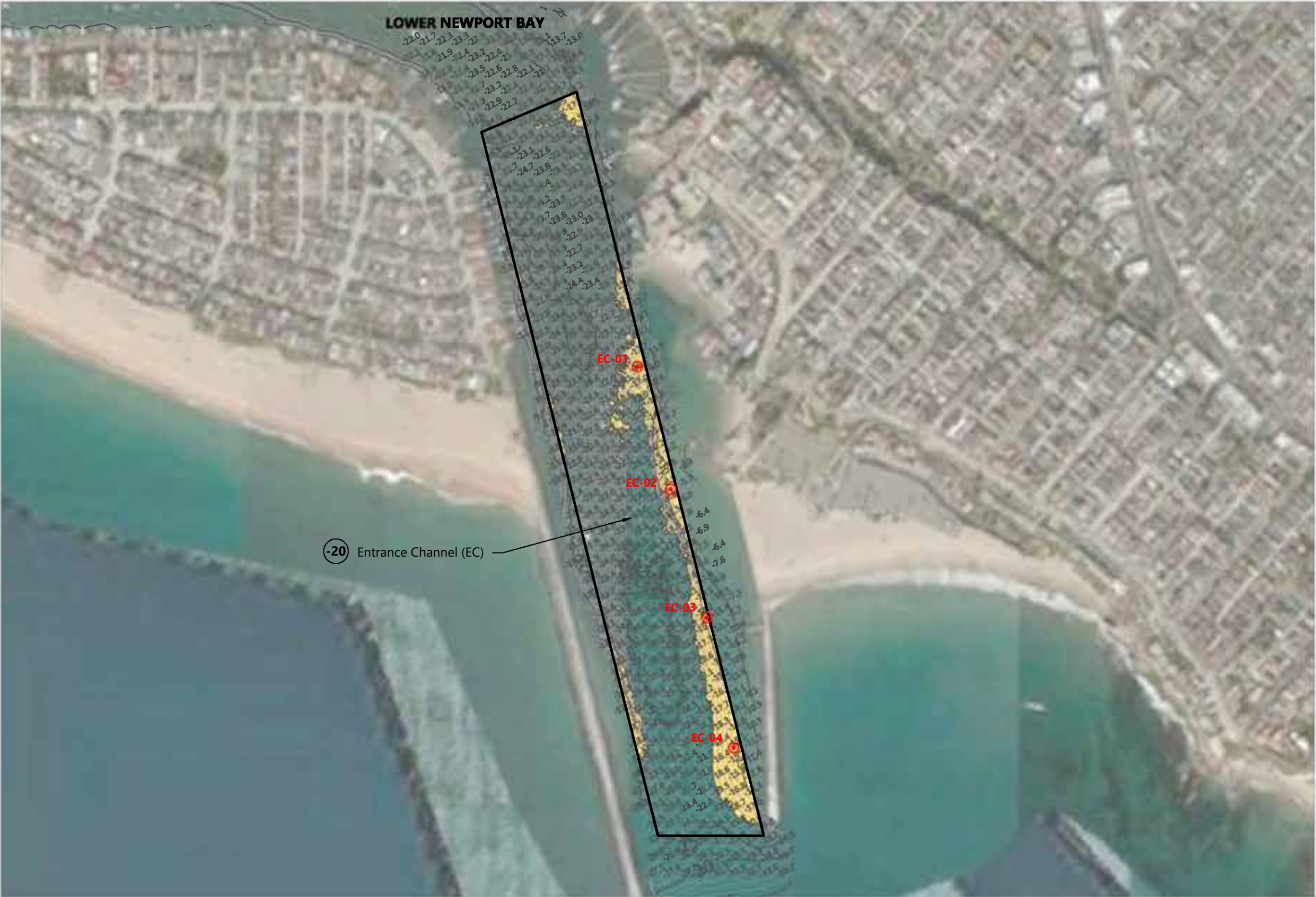
Figure 15 Dredge Unit, Bathymetry, and Actual Sampling Locations - Entrance Channel Lower Newport Bay Federal Channels Dredging
