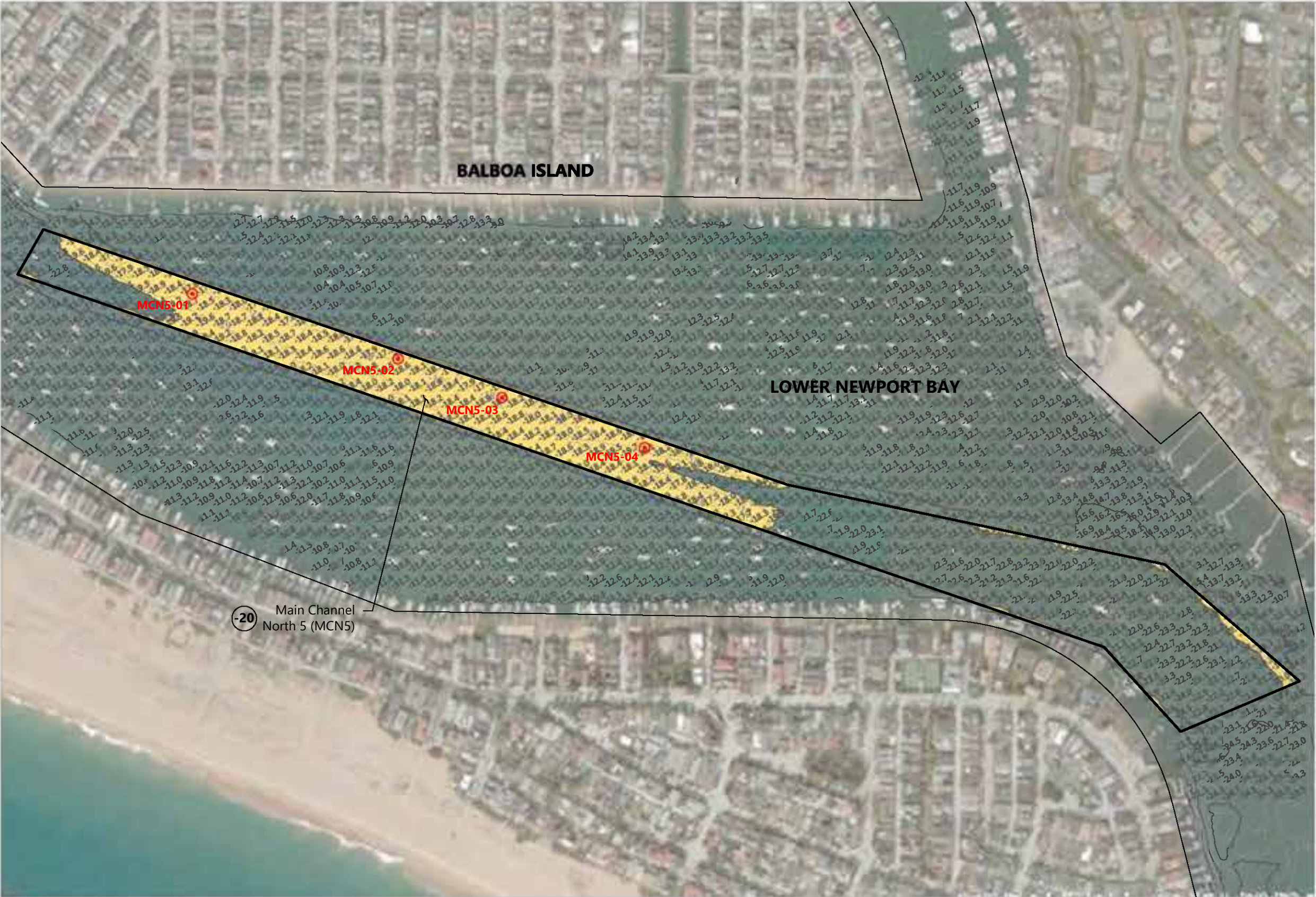
Figure 10 Dredge Unit, Bathymetry, and Actual Sampling Locations - Main Channel North 5 Lower Newport Bay Federal Channels Dredging
