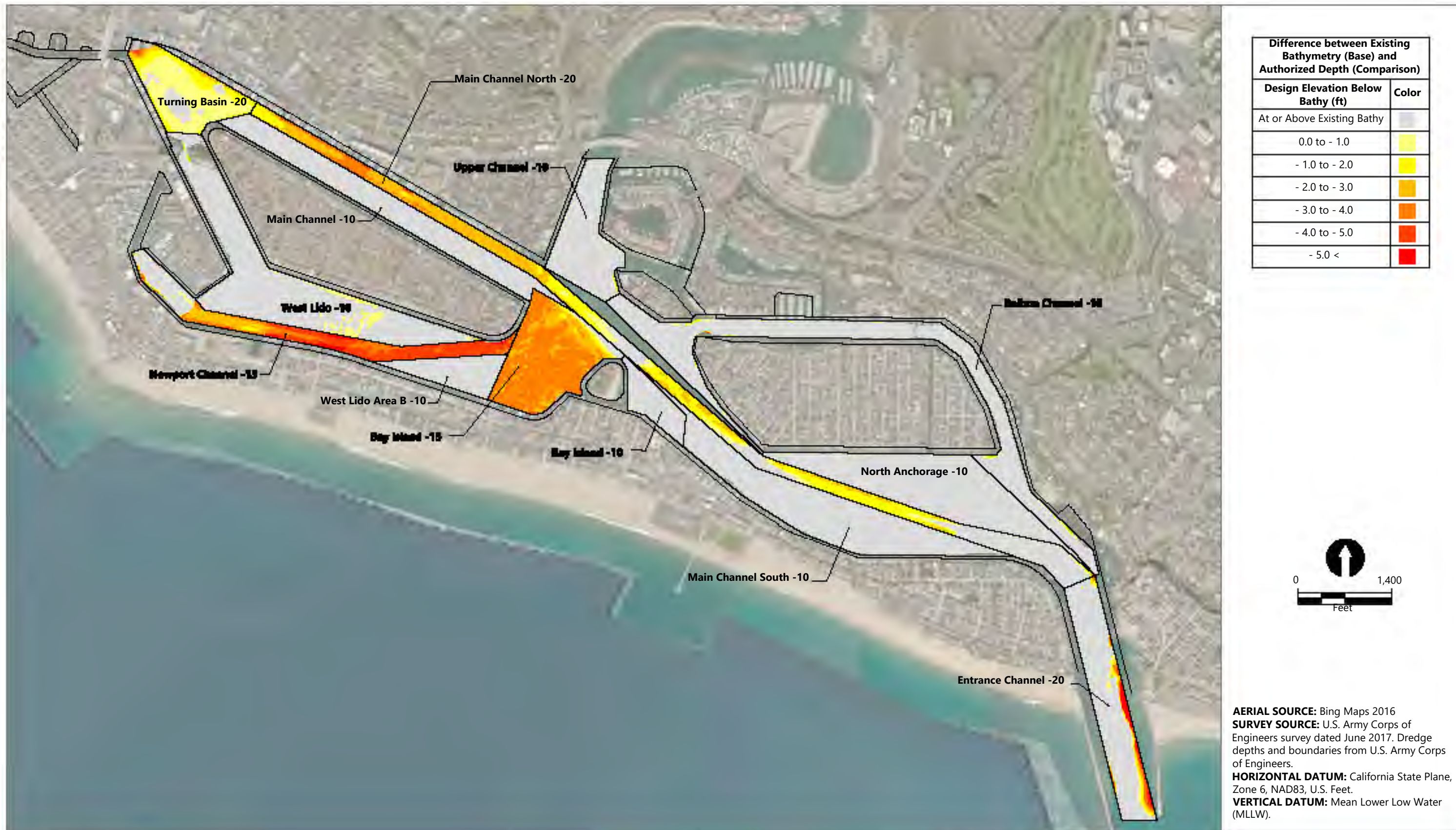
Figure 3 Comparison of 2017 Harborwide Bathymetric Survey to Authorized Design Depths Lower Newport Bay Federal Channels Dredging
