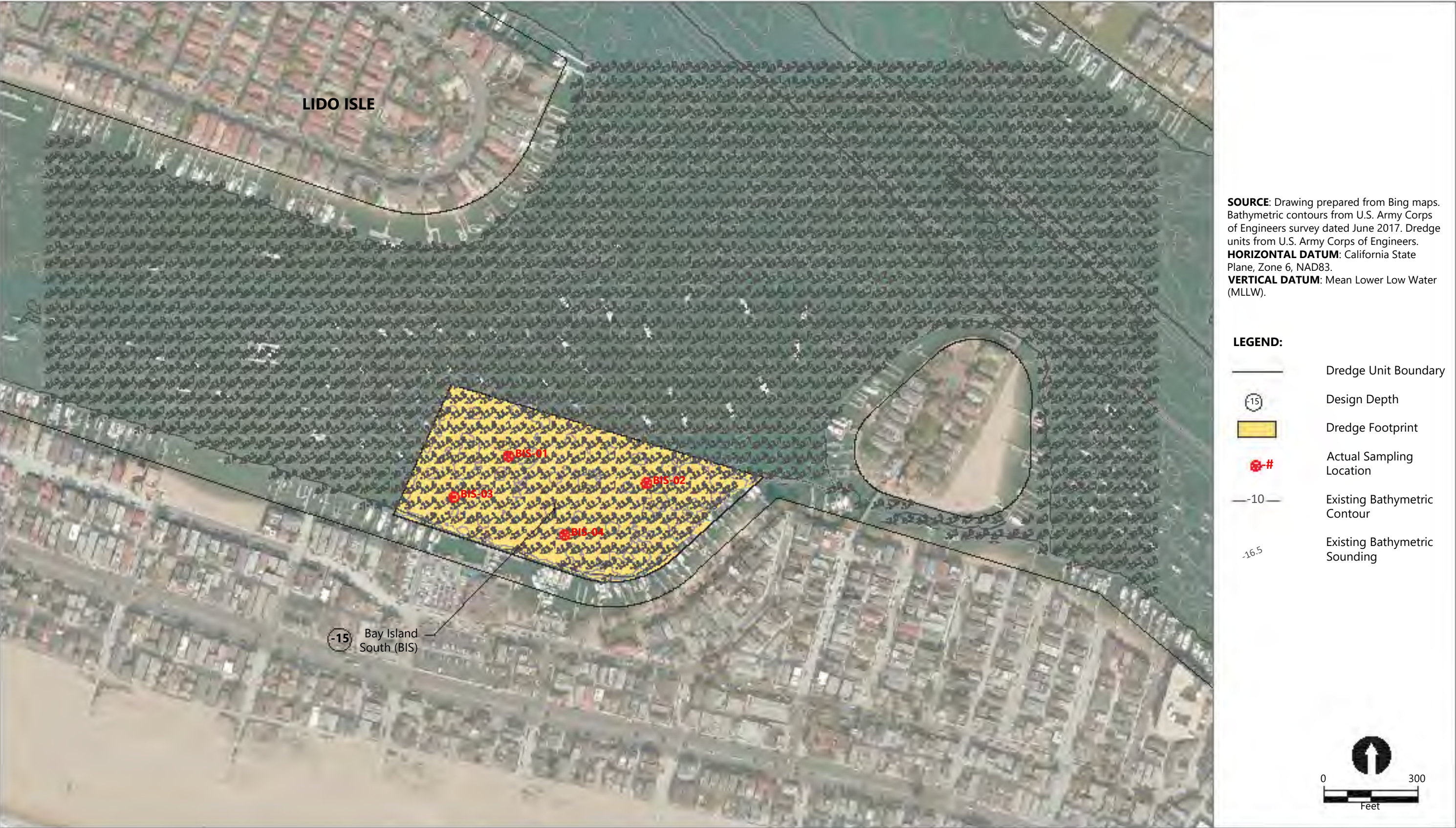
Figure 14 Dredge Unit, Bathymetry, and Actual Sampling Locations - Bay Island South Lower Newport Bay Federal Channels Dredging
