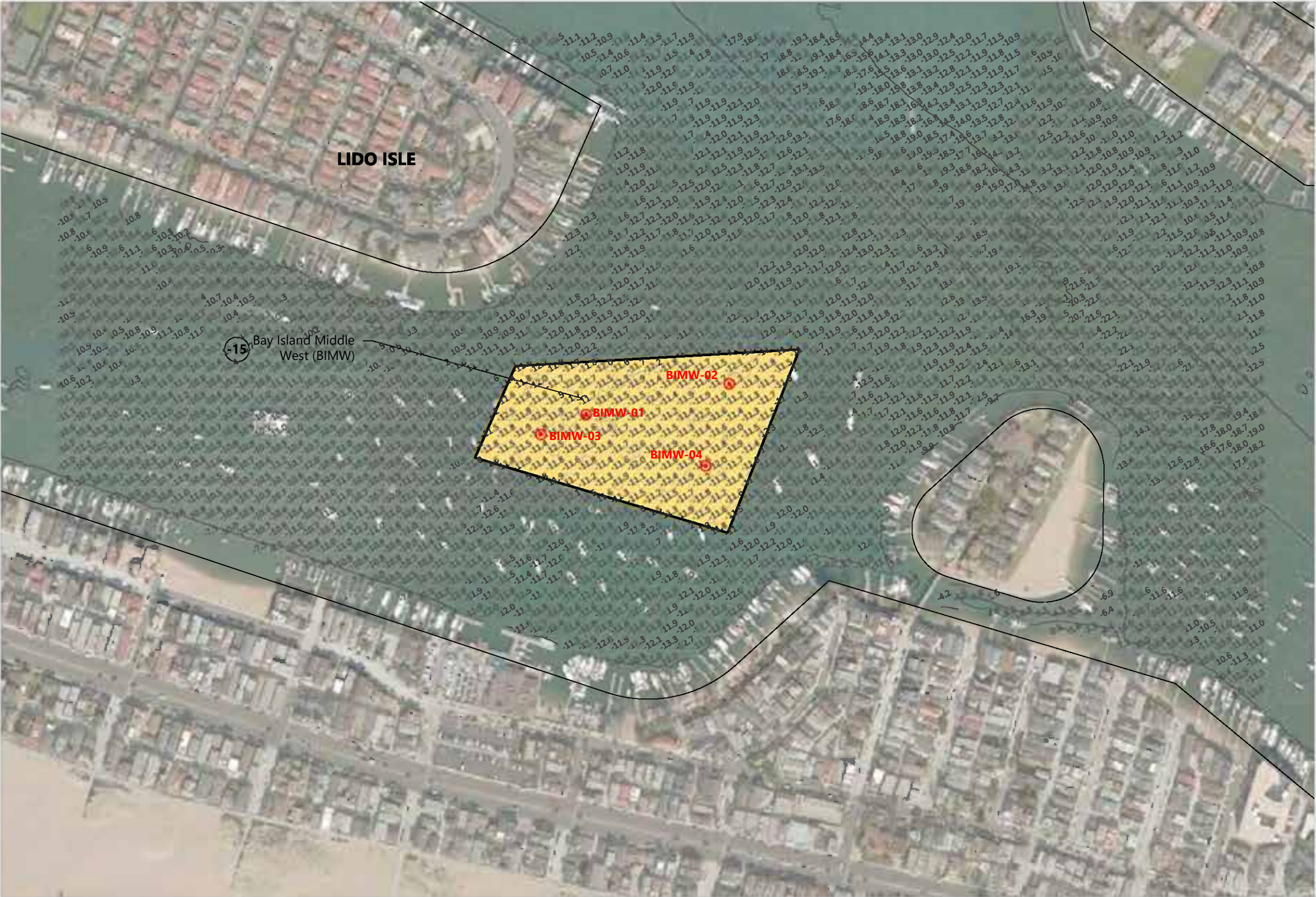
Figure 13 Dredge Unit, Bathymetry, and Actual Sampling Locations - Bay Island Middle West Lower Newport Bay Federal Channels Dredging
