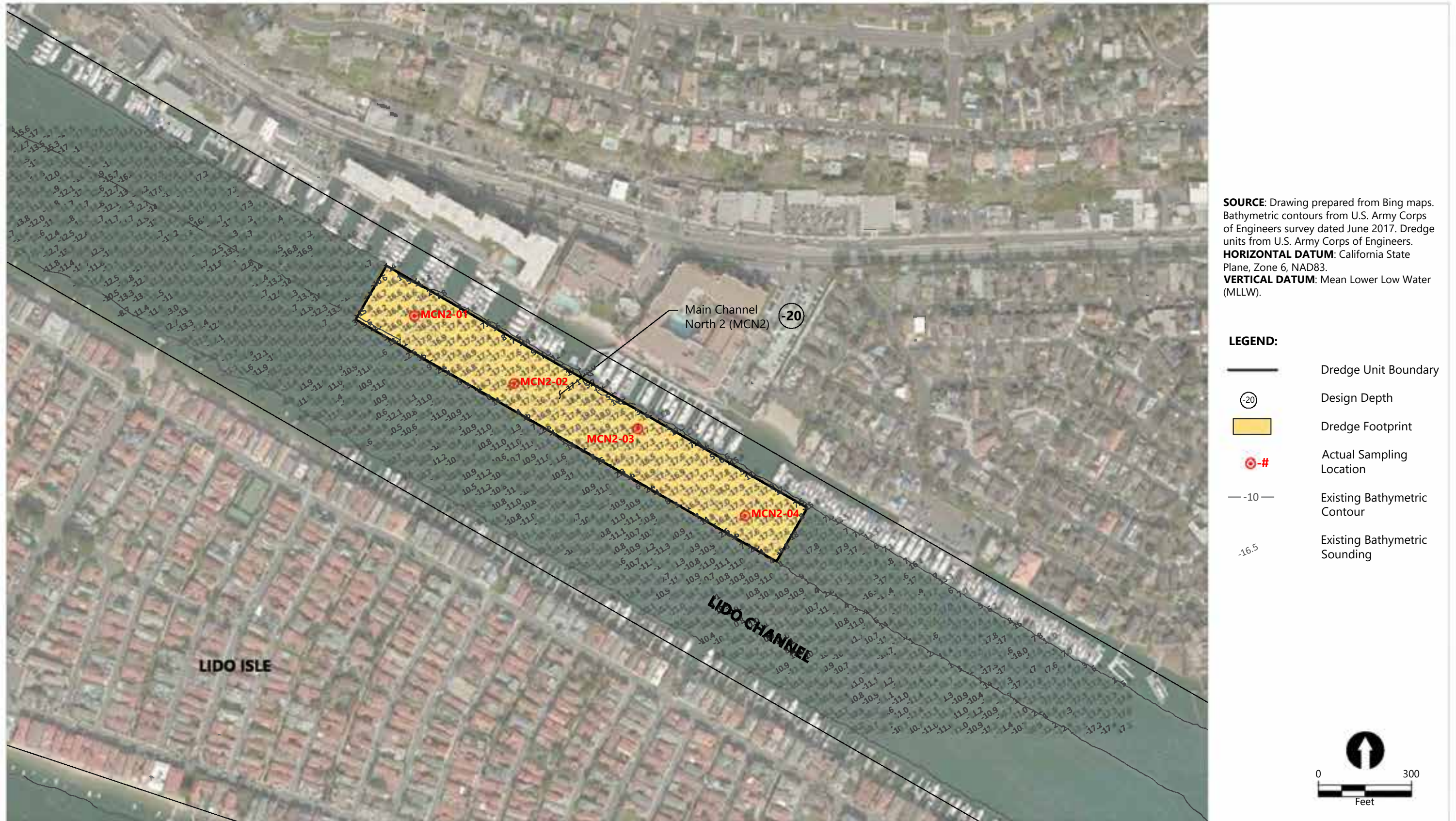
Figure 7 Dredge Unit, Bathymetry and Actual Sampling Locations - Main Channel North 2 Lower Newport Bay Federal Channels Dredging
