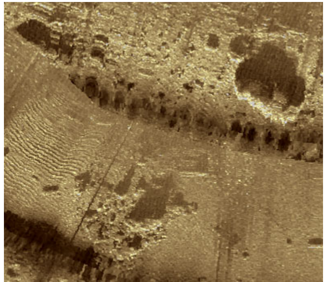
Example interferometric sidescan image of the bottom within the Point San Luis Survey Area. The image illustrates rock bottom habitat of low and high relief reef along with sand bottom and energy influenced sand bottom, represented by the sand ripples.
