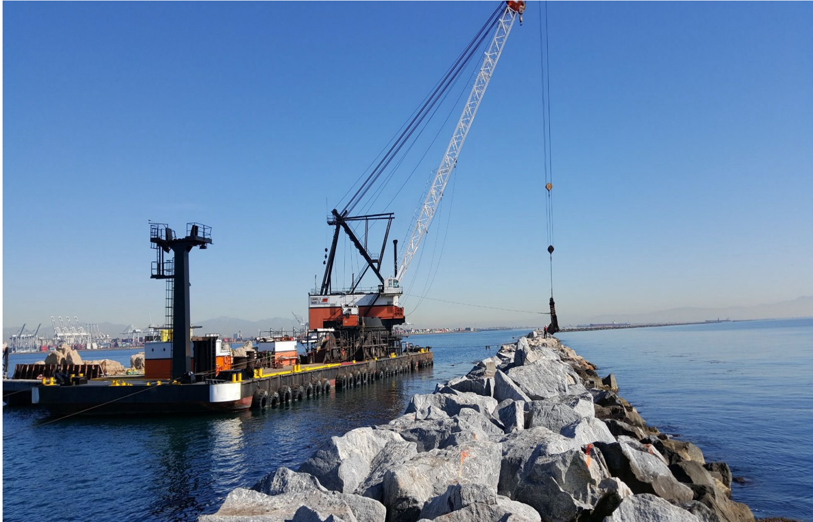
Figure 5: Example photo of crane-equipped barge which is utilized for breakwater repair.
