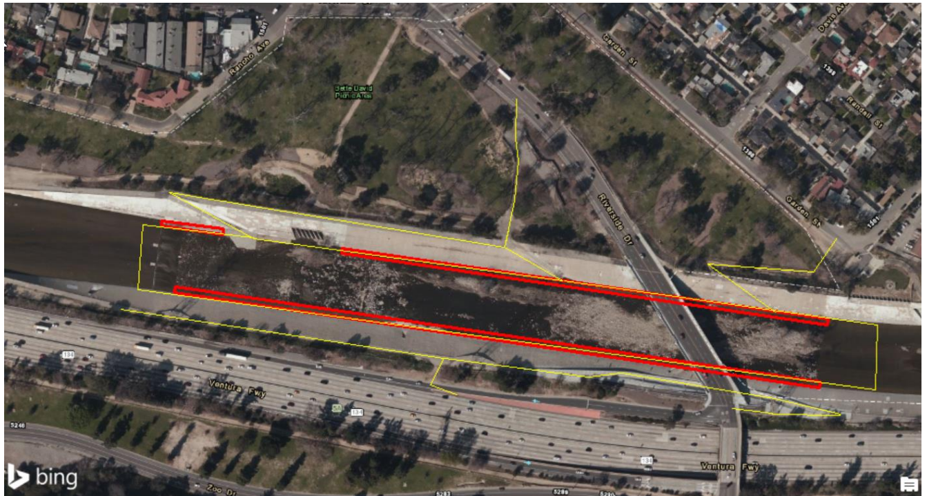
Figure 2: Construction vehicle routes in and out of the channel are noted by the yellow lines. Red outlines are the repair areas.
