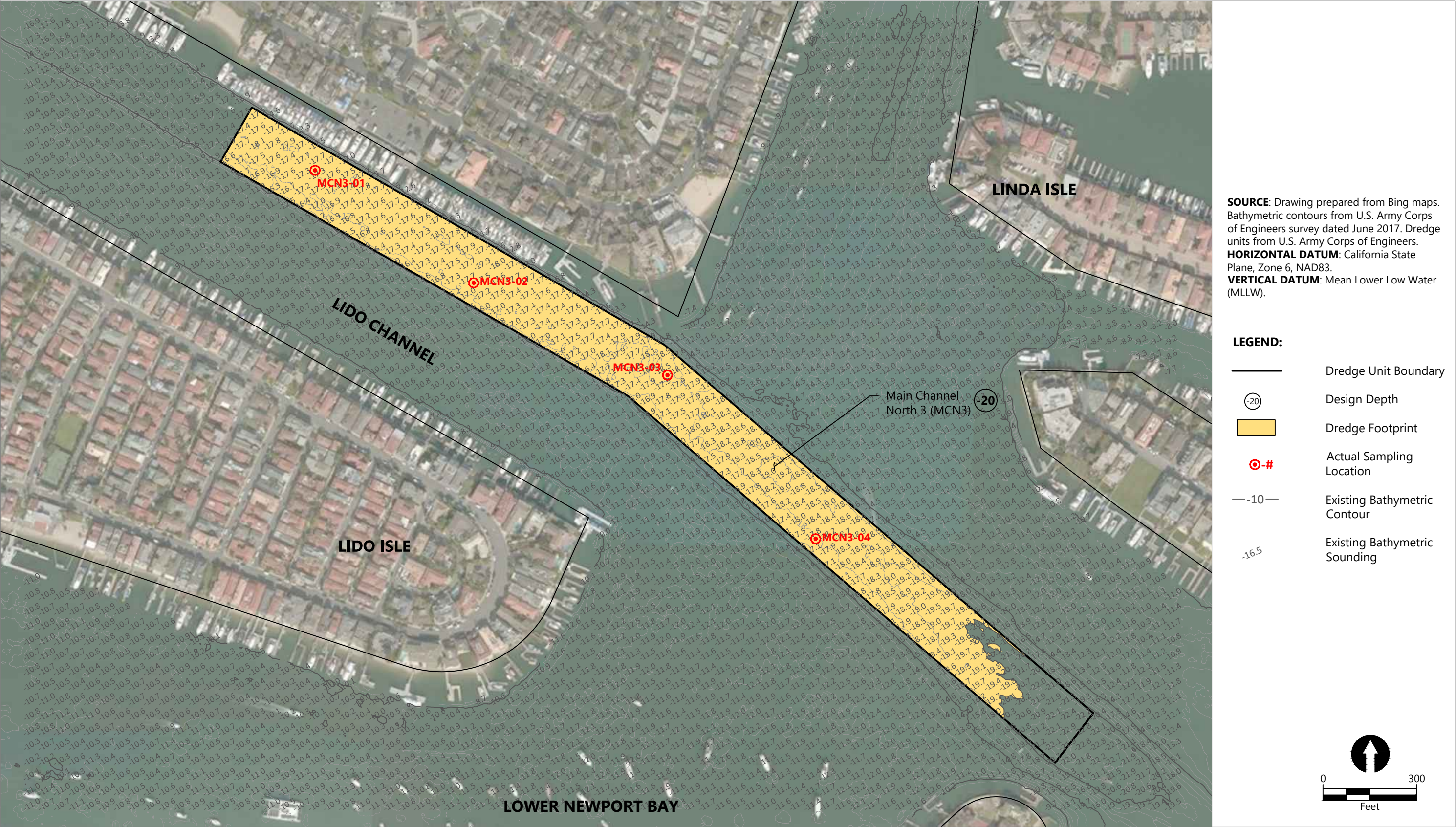
Figure 8 Dredge Unit, Bathymetry, and Actual Sampling Locations - Main Channel North 3 Lower Newport Bay Federal Channels Dredging
