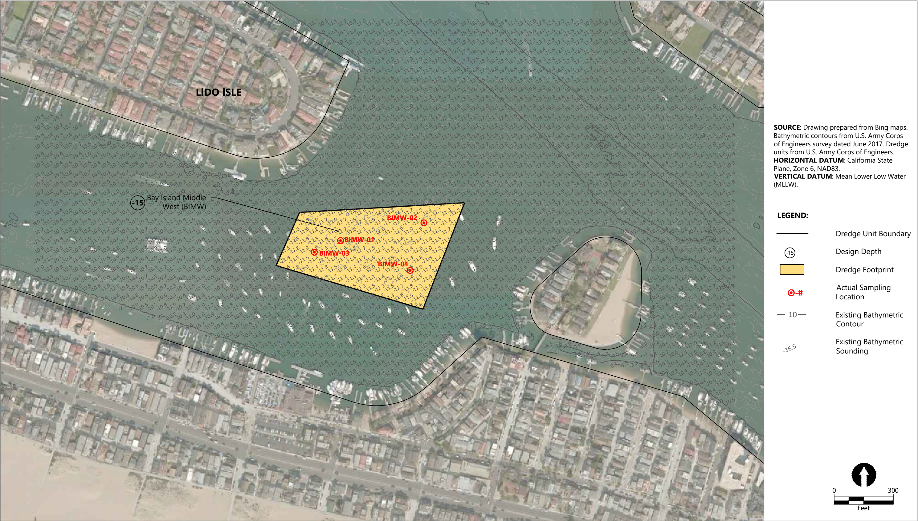
Figure 13 Dredge Unit, Bathymetry, and Actual Sampling Locations - Bay Island Middle West Lower Newport Bay Federal Channels Dredging
