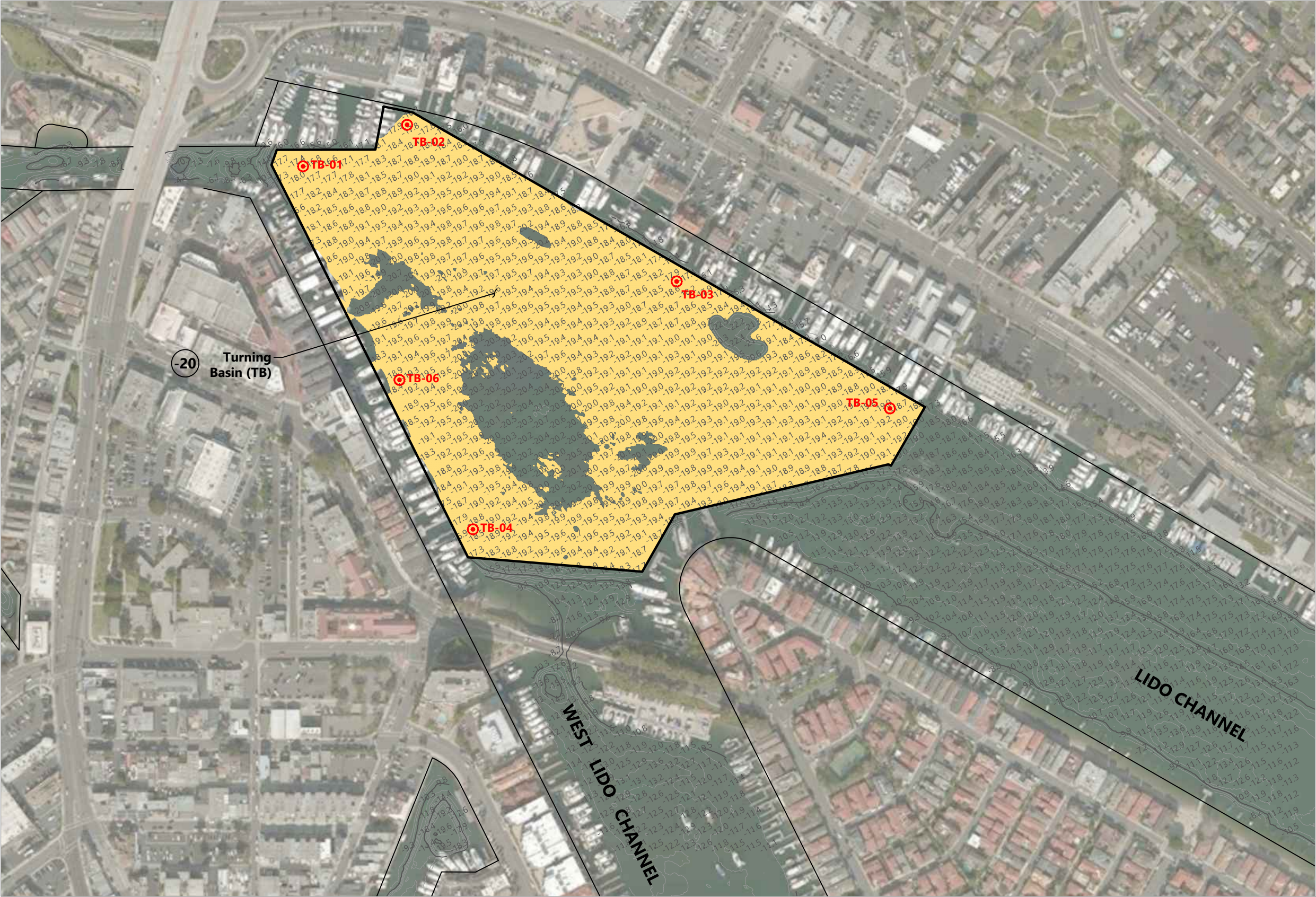
Figure 5 Dredge Unit, Bathymetry, and Actual Sampling Locations - Turning Basin Lower Newport Bay Federal Channels Dredging
