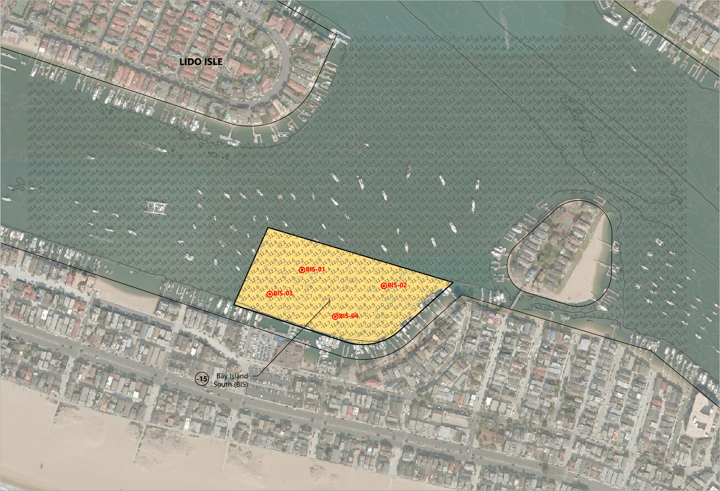
Figure 14 Dredge Unit, Bathymetry, and Actual Sampling Locations - Bay Island South Lower Newport Bay Federal Channels Dredging
