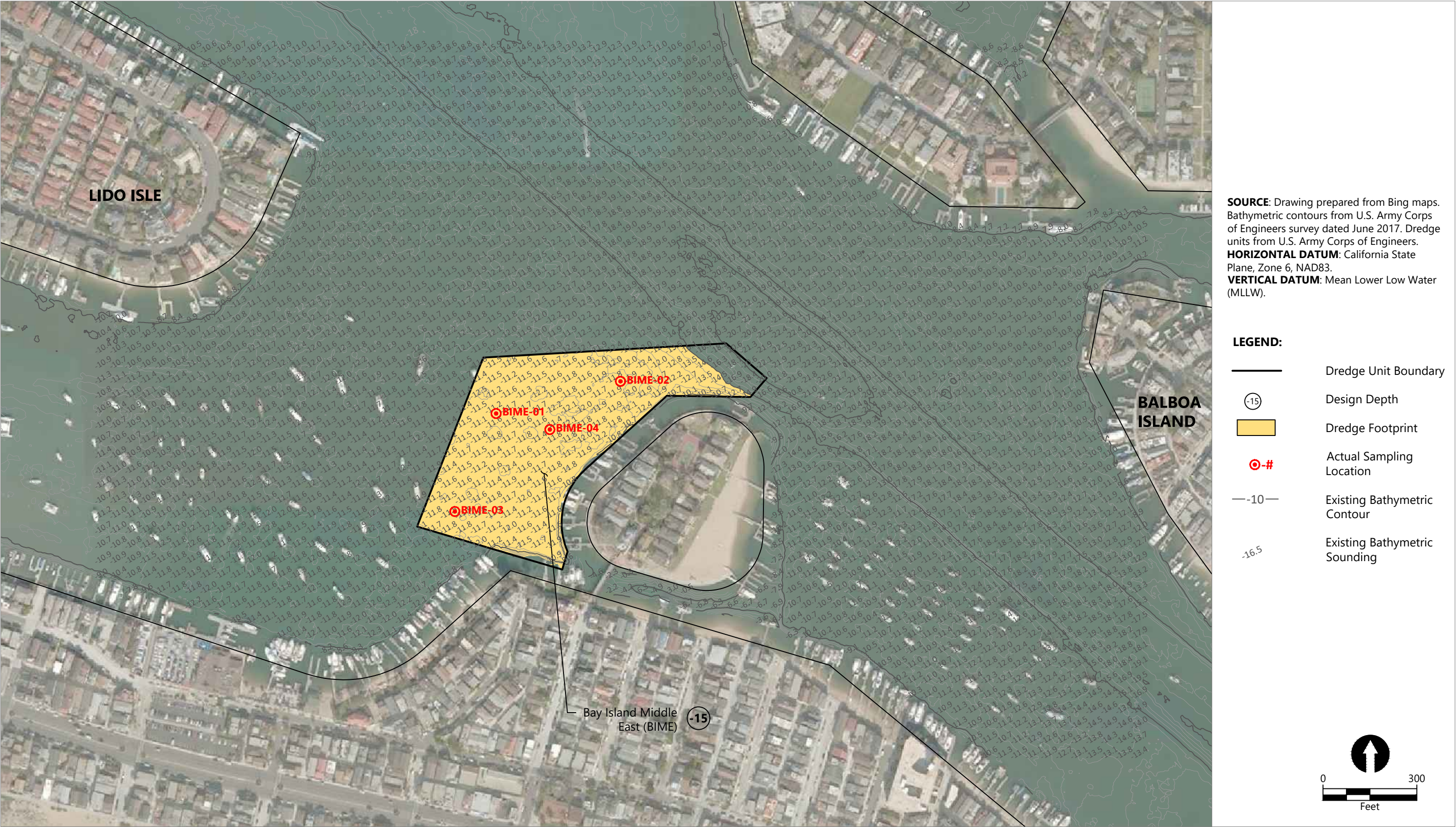
Figure 12 Dredge Unit, Bathymetry, and Actual Sampling Locations - Bay Island Middle East Lower Newport Bay Federal Channels Dredging
