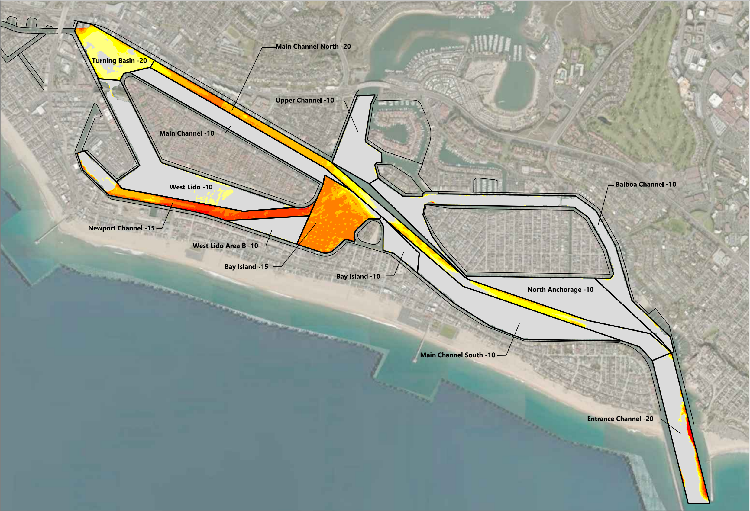
Figure 3 Comparison of 2017 Harborwide Bathymetric Survey to Authorized Design Depths Lower Newport Bay Federal Channels Dredging
