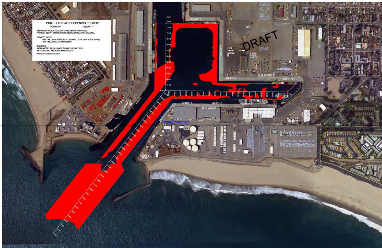
Figure 8. Port Hueneme Federal Channels. Red areas require dredging, remaining areas are at project depth or below and do not require dredging. Slope protection shown as blue line.
