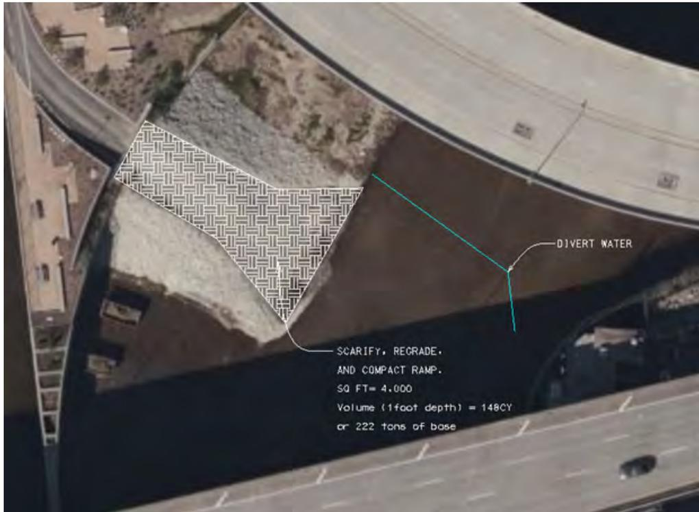
Figure 2: Proposed repairs.
