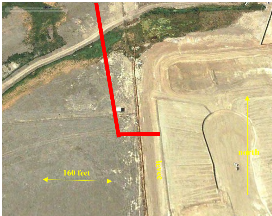
Fig. 36.—2007 view of south end, conceptual River Road Dike alignment (approximated by red line). Note housing pad grades up and into the pre-existing levee slope. Photo from Google Earth Pro.
