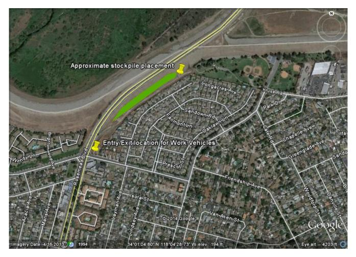
This aerial photograph indicates general areas, proposed for access off Rosemead Blvd. and for placement of sand and gravel, for the purpose of prepositioning materials on Corps land in advance of potential short-term needs in the future for flood risk management and maintenance activities.
