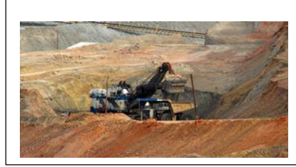
Shovel loading a truck at Ray Mine.
