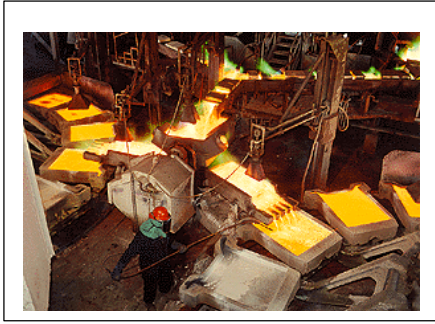
Copper being poured into anode molds.
