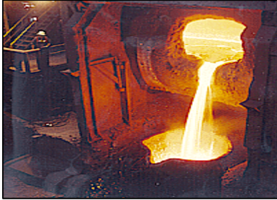
Blister copper being poured from the converter furnace.
