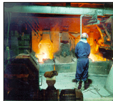
Matte being tapped from a hole at the bottom of the oxygen flash furnace.
