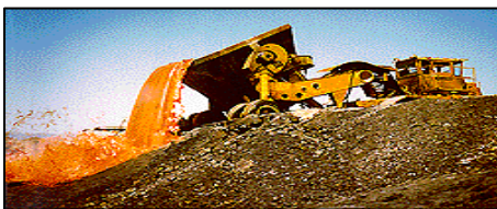
Slag being dumped to cool. The pouring of slag resembles a man-made lava flow and can be quite spectacular at night.
